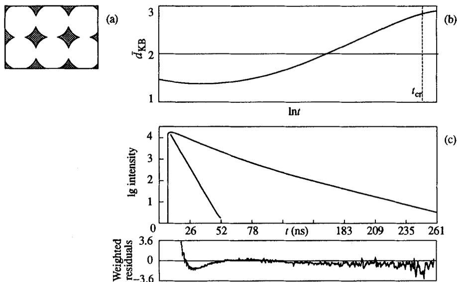
FIGURE 3 (a) Mashed spheres. (b) Apparent dimension versus  $\ln t$  for the mashed spheres model. ( $d_{FA} = 3.278$ ,  $\chi^2 = 0.427$ ).
