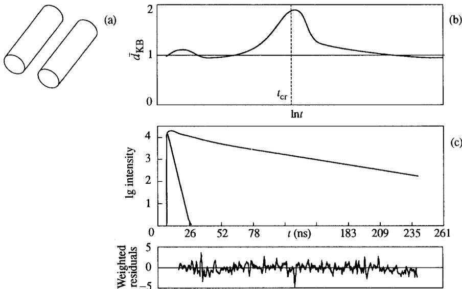
FIGURE 2 (a) Parallel cylinders. (b) Apparent dimension versus  $\ln t$  for the parallel cylinders model. (c) Simulated lamp and donor decay functions for the parallel cylinders model. ( $d_{FA} = 2.076$ ,  $\chi^2 = 1.818$ ).
